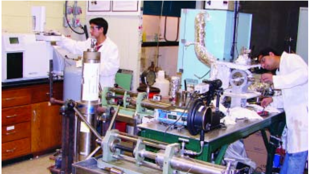
A state-of-the-art Gas Chromatograph (left) is being operated by PETE undergraduate student Mauricio Toscano, and the high-pressure optical cell is being assembled for gas-oil interfacial tension measurement by PETE graduate student Daryl Sequeira.
