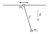
The pendulum ( $m_2$ ) pictured is subject to gravity and is attached to a slider of mass  $m_1$  which can, without friction, move in the horizontal directions.
