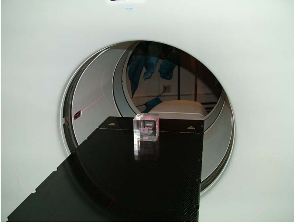
Figure 6. Phantom aligned with positioning lasers prior to image acquisition.
